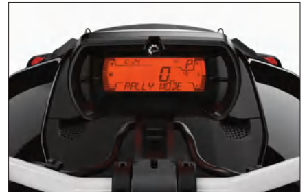
RALLY MODE AND TIRES Allows you to have more flexibility and fun off-pavement by optimizing VSS input and enabling you to perform controlled drifts with adapted all-road tires.
